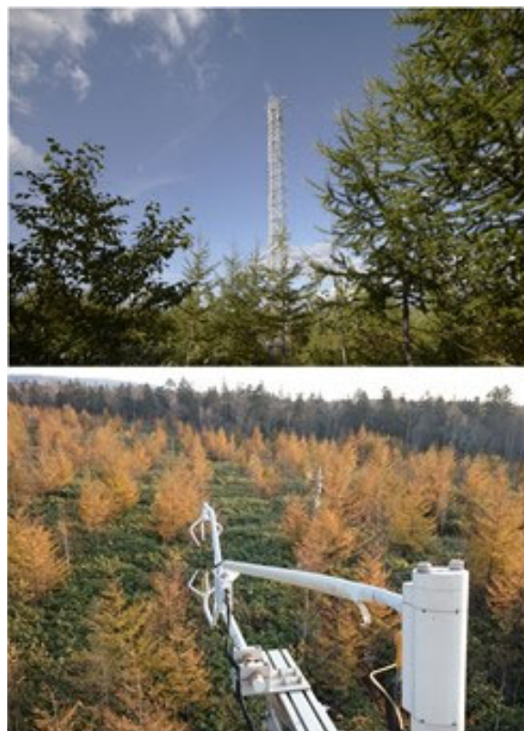
Figure 2. 30-m high CO 2 flux monitoring tower (upper) and sensors (lower)
